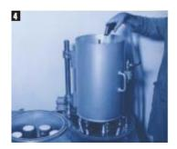
**4.** To clean the machine the mixer is swivelled over the drain bowl and then cleaned with a spray nozzle. The stirring unit is hereby raised by 100 mm using a compressed-air cylinder.
