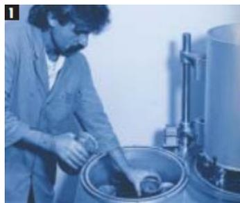
**1.** 8 flasks are placed in the mixer and the stirring unit is swivelled over them.
