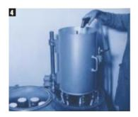
**4.** To clean the machine the mixer is swiveled over the drain bowl and then cleaned with a spray nozzle.
