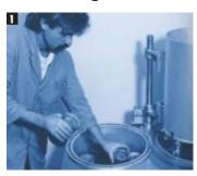
**1.** 6 flasks are placed in the mixer and the stirring unit is swivelled over them.
